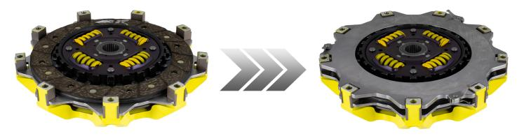
Line up the second friction plate onto the drive gear with "TRANS SIDE" facing down.
